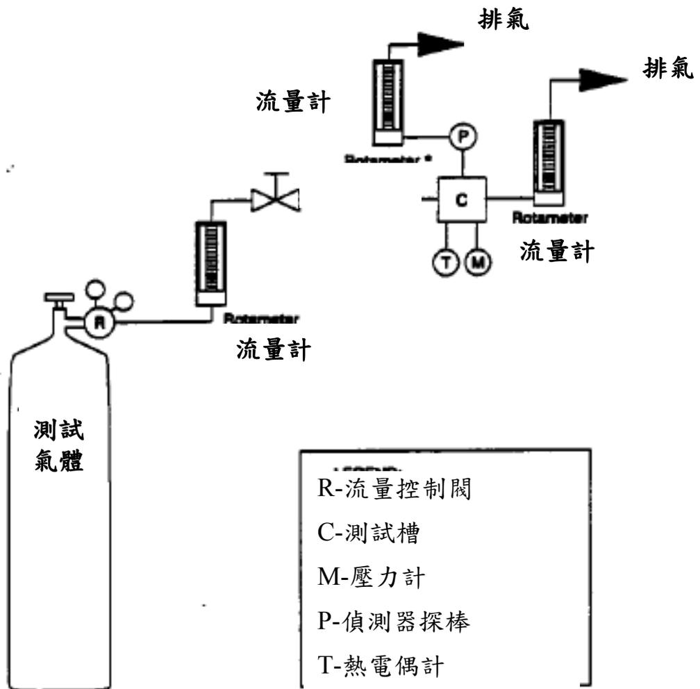
備註：以”Accuracy and Response Time for Vapor-phase Out-of-Tank Petroleum Detectors”及”Specificity for Vapor-phase Out-of-Tank Petroleum Detectors”為例
