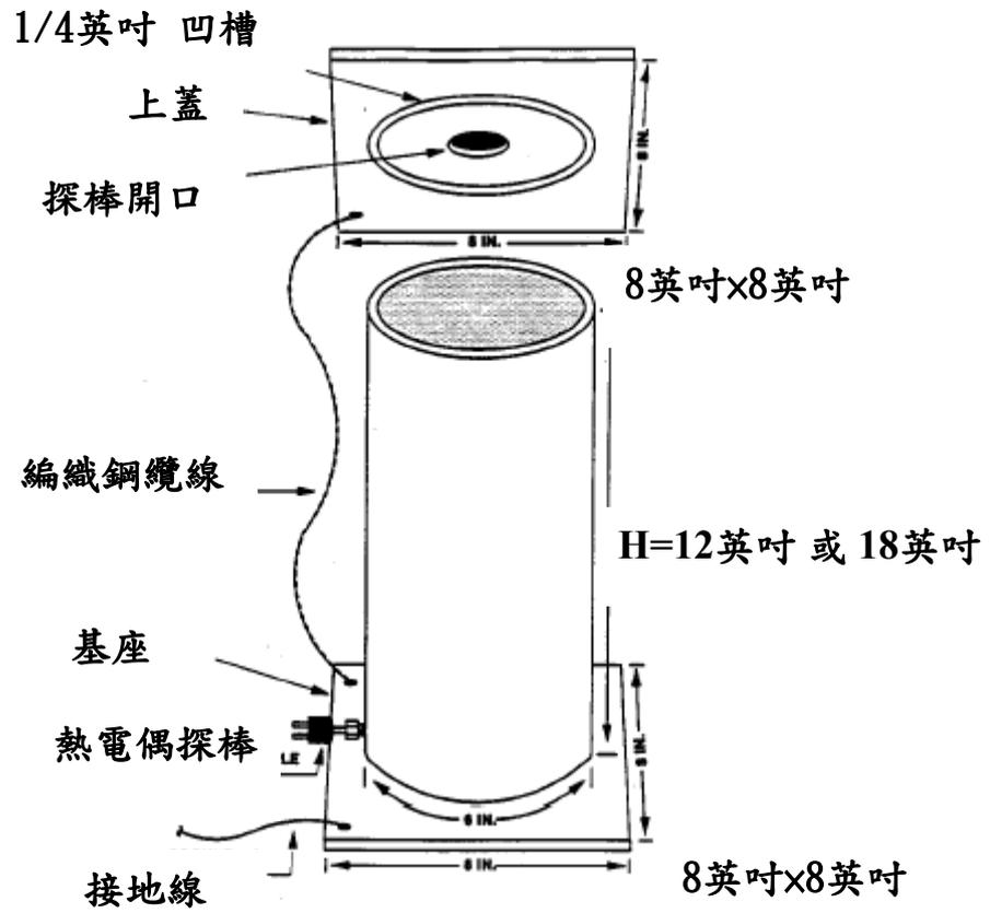
圖3 液相儲槽外偵測器(Liquid -phase Out-of-Tank Product Detector) 滲漏
